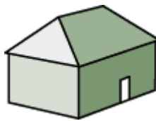
Simple A hipped roof where all four roof faces rise to a ridge across the top, often with broader faces across the front slope and narrower side sections.
