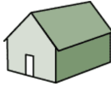
Front-gabled houses have the peak or gable facing the front.
